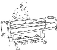
5. With the foot control the nurse can adjust the bed to the horizontal position, place the patient on his back, place the other siderail in an erect position and place a pillow against it for the patient.
